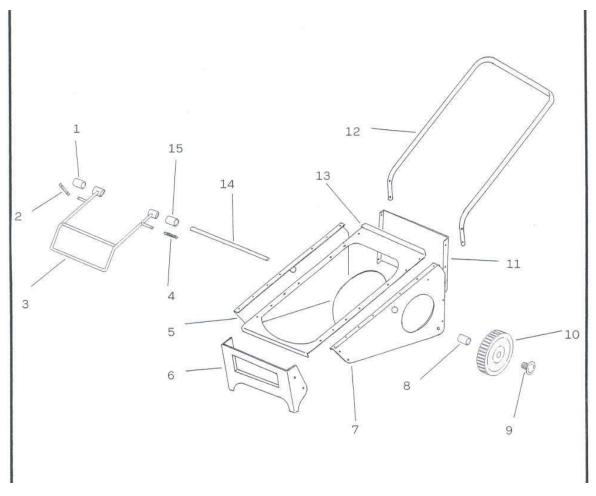
To remove the drum from this frame it is necessary unscrew the frame parts No. 13 and 5 first. To remove the yellow hose from the drum to can change the drum support No. 17 and 18.
